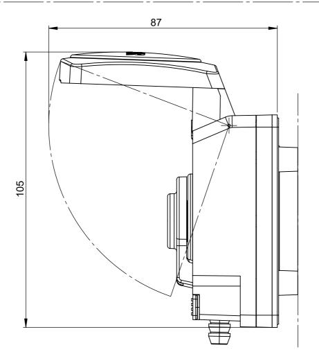
Open pump is examplary visualization based on 15KU with NEMA23 as 3 Roller Version (#15701.300) with Single 6.4x1.6 Straight Tube Set (#15000.228). Dimensions of open pump valid for all pumps of 15KU family.
