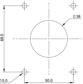
fixation with ISO 7045 - M4 or similar max. head diameter 8.0, max. height 3.5 min. thread length 10 + Panel Thickness
