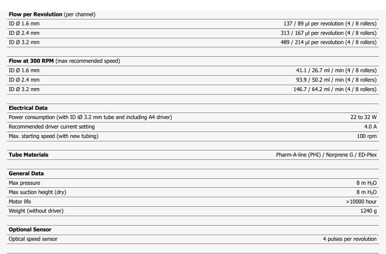
All data measured with 'run-in' Pharm-a-line tubing and  $H_2O$ .
