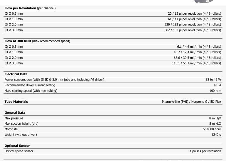
All data measured with 'run-in' Pharm-a-line tubing and  $H_2O$ .
