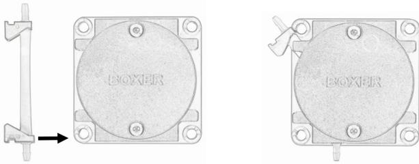
**2** Push the upper tube clip into the recess in the pump body. Some tension in the tube will be required as it is pulled over the rollers.
