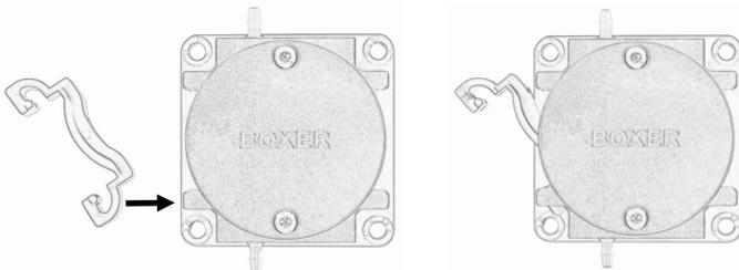
**4** Push the upper end of the saddle down, rotate the saddle and insert the upper pin of the saddle into the recess in the pump.
