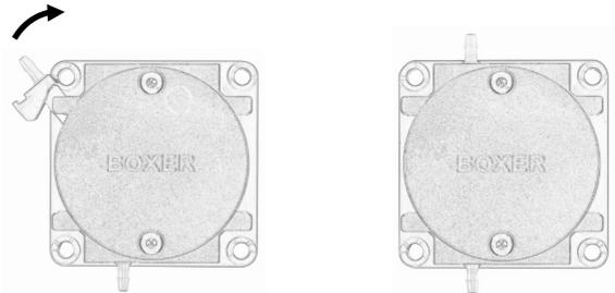
**3** Align the saddle with the pump body in the orientation shown below. Insert the lower pin of the saddle into the recess in the pump body.
