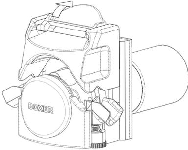
❷ Remove the M3x12mm screw. Close clamp lever.
