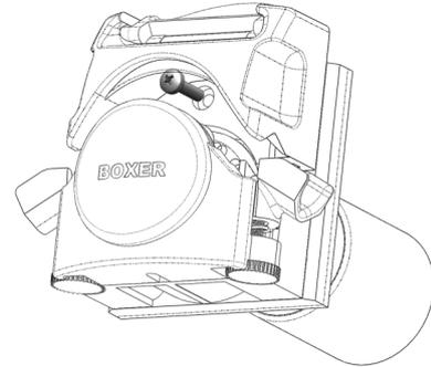
❸ Push head lock lever in direction on the motor. Rotate the head anti clockwise.
