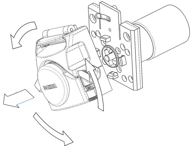
❺ To re-assemble: open tube clamp lever. Align head with motor plate at the angle shown below. Rotate pump rotor until the rotor is aligned with drive pin. Push head into bayonet.
