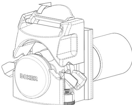
The tube grips are sprung loaded and adjust automatically to the OD of the tube. The 15QQ is designed for 1.6 mm wall tubing from ID of 1.6 to 4.8 mm. Only tubing suitable for peristaltic pumps should be used.
