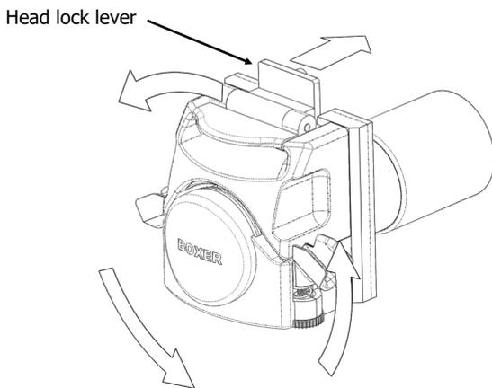
❹ Pull the head assembly away from the motor plate.
