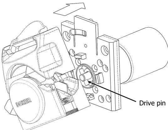
❻ Rotate head assembly clockwise until 'clicks' into position. Replace M3x12mm screw. Close tube clamp lever.
