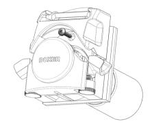
4 Pull the head assembly away from the motor plate.
