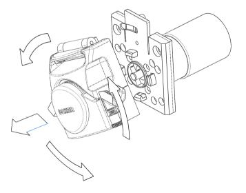
S Rotate head assembly clockwise until 'clicks' into position. Replace M3x12mm screw. Close tube clamp lever.
