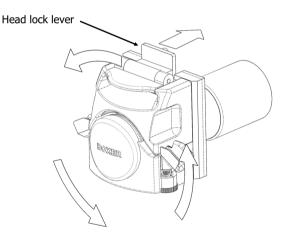
**⑤** To re-assemble: open tube clamp lever. Align head with motor plate at the angle shown below. Rotate pump rotor until the rotor is aligned with drive pin. Push head into bayonet.
