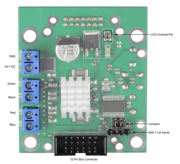
5.1 Analogue Mode Inputs In analogue mode the following inputs / outputs are used via the 12 pin box connector:
